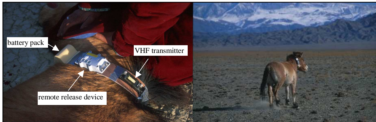
Fig. 1: North Star ® GPS / ARGOS collar during mounting (left) and on a standing Przewalski horse (left) in Takhin Tal, Mongolia.
